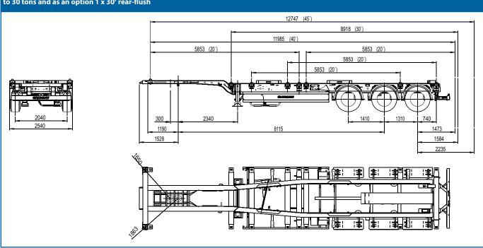
Attention: Transport of filled tank container is not allowed! Container position 20' in centre position limited to 30 tons. During transport of 45' containers with short tunnel the allowed length from the king pin to the rear is exceeding legal limits! The transport of 45' containers with long tunnel and chamfered corners at front is possible within the EC directive. The rear bumper must be pulled out manually!
